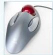
The Trackball Mouse Lets you control the cursor with your fingers or hands instead of needing to move the wrist or arm.
